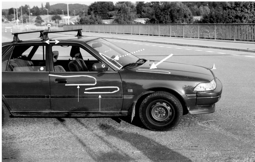
FIG. 1—Car damages: a) impact point of the left hip region (thick arrow); b) impact point of the left trunk (dotted arrow); c) car roof girder was dislocated 20 cm backwards (double arrow); and d) scrub marks on the right front door of the car caused by bicycle (two thin arrows).
